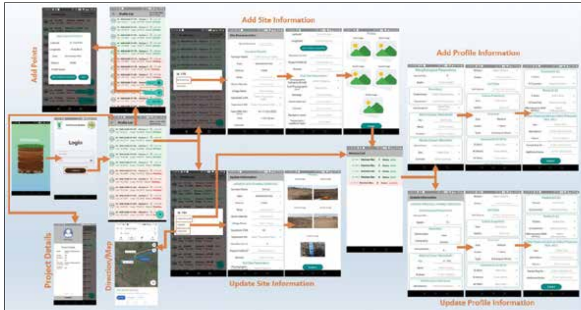
Fig. 2.6.4. Workflow of MobileApp on 'Soil Survey Data Collection and Management System (SDCMS)
