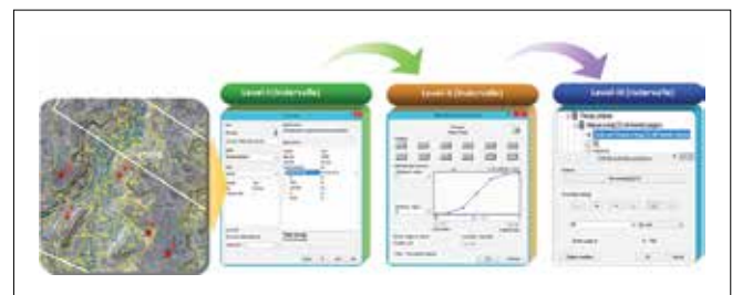
Fig. 2.2.10 : Hierarchical object based segmentation algorithm process for generating LEU maps
